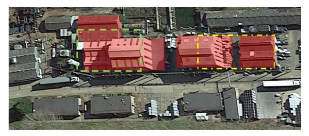
The new warehouse will occupy the space outlined in yellow and will be 9m to the eves and have a floor area of no more than 800m<sup>2</sup>. The remaining area will be returned to hardstanding / simple low level covered storage (area indicated by the green dotted outline).
