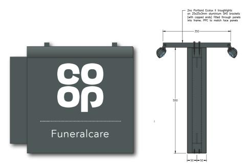
1No. Externally illuminated Projector sign. RAL 7010 with white applied vinyl lettering. Consisting of 2mm folded aluminium panels having 50mm returns fitted back to back around steel support framework, with mild steel projecting arms and fixing plate, being powder coated RAL 7010. **Size:** 550mx550mm
