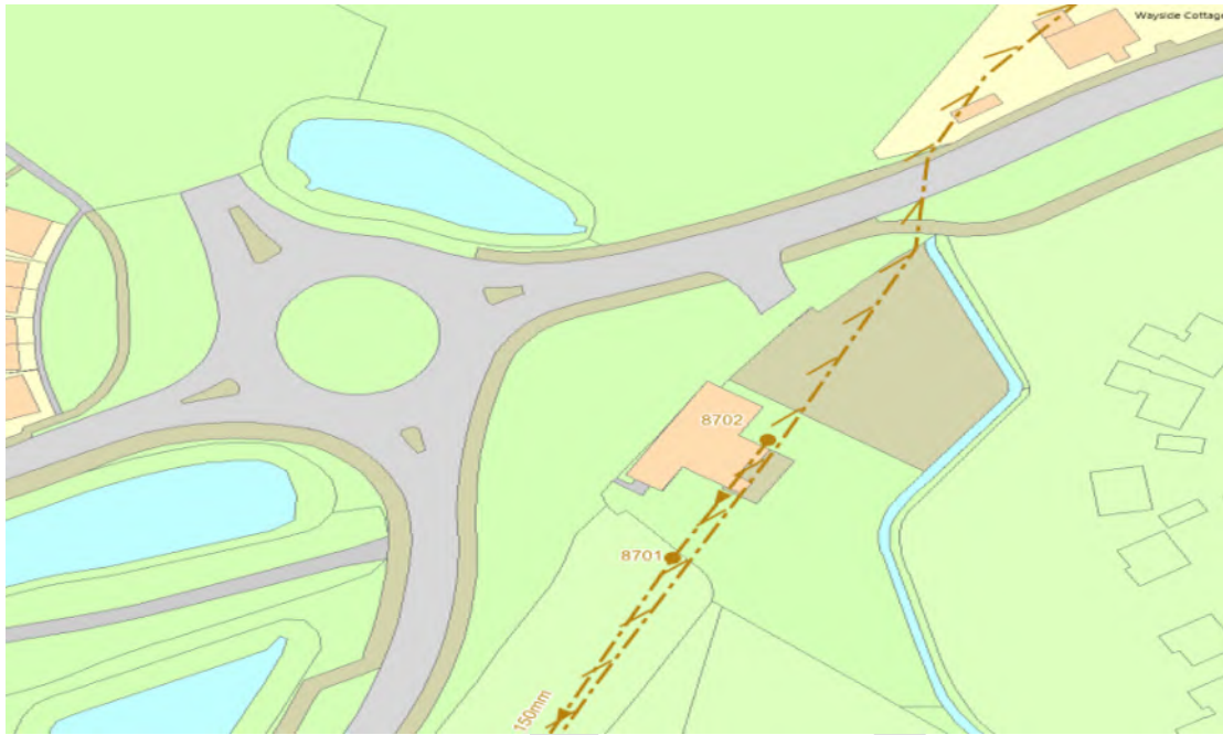
Figure 3.3: Foul and Rising Main Diversion Required
