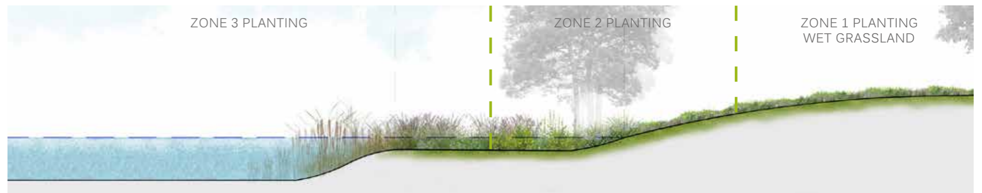
Figure 23. Cross section through SUDS planting
