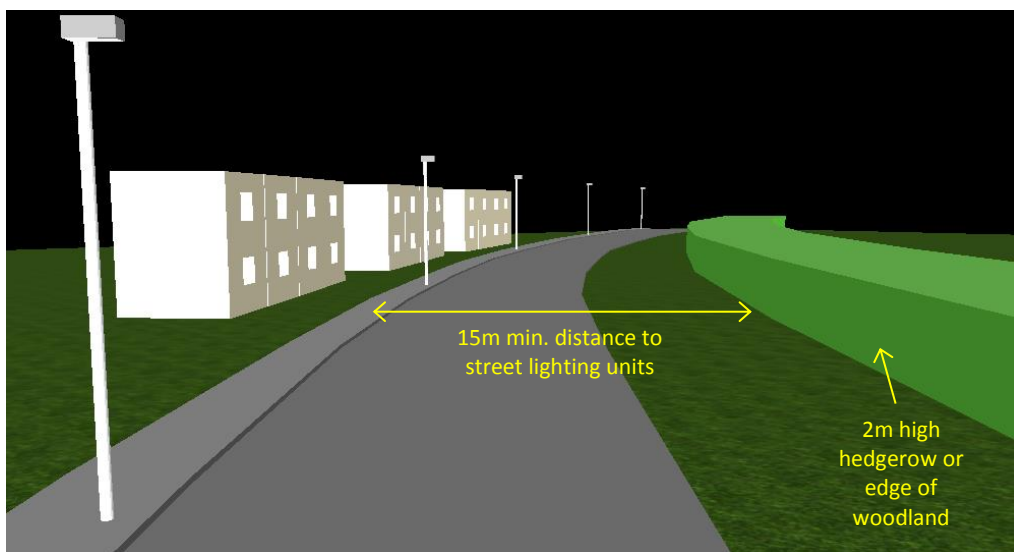
Figure 2a: Street lighting arrangement near bat routes
