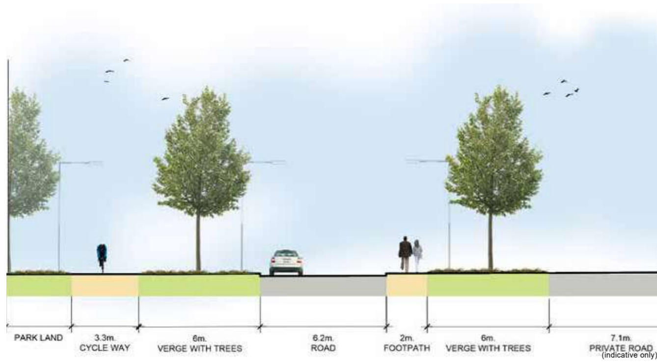
Figure 19. Section A - Northern End of the Spine Road Showing Wide Verges (Parkland Edge)
