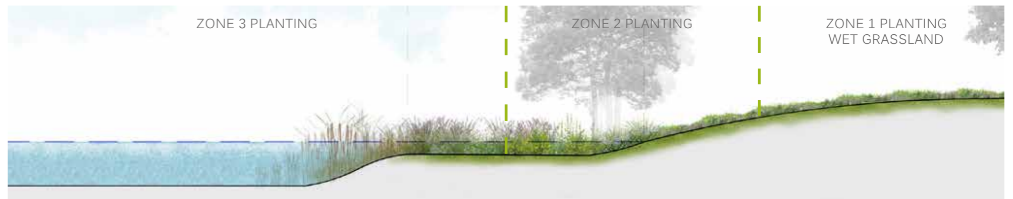
Figure 23. Cross section through SUDS planting
