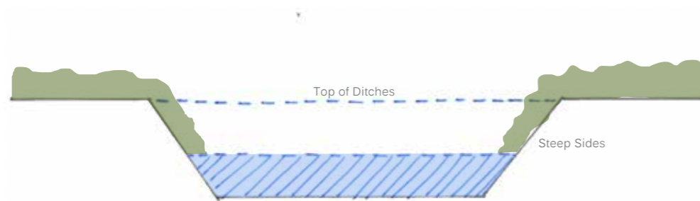
Figure 14. Typical Section Through Existing Drainage Ditch
