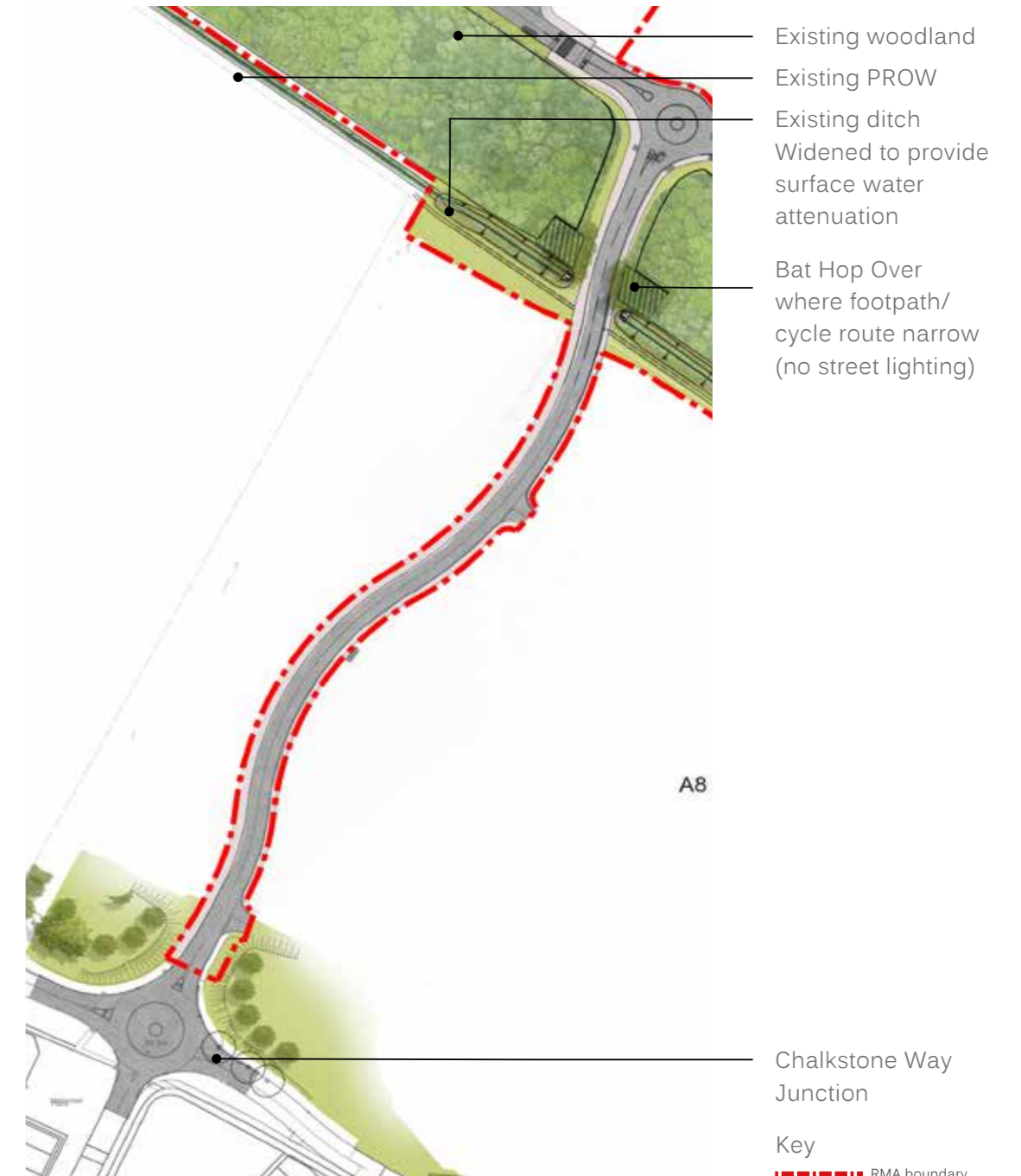
Figure 11. Detail Area: Southern Road Verges
