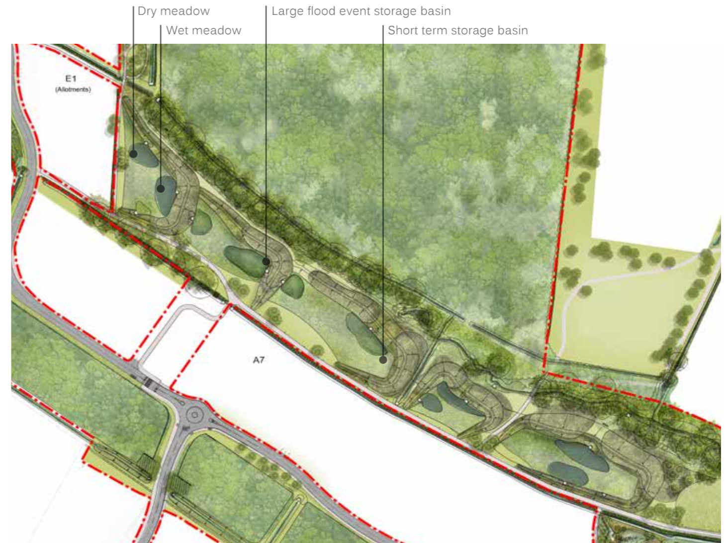
Figure 17. Stormwater Basins Extract from General Arrangement Plan
