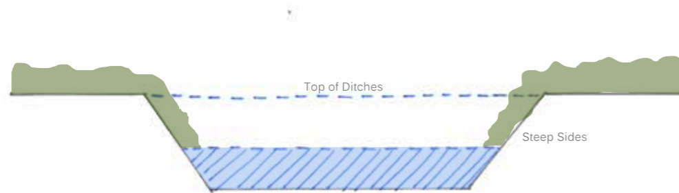
Figure 14. Typical Section Through Existing Drainage Ditch
