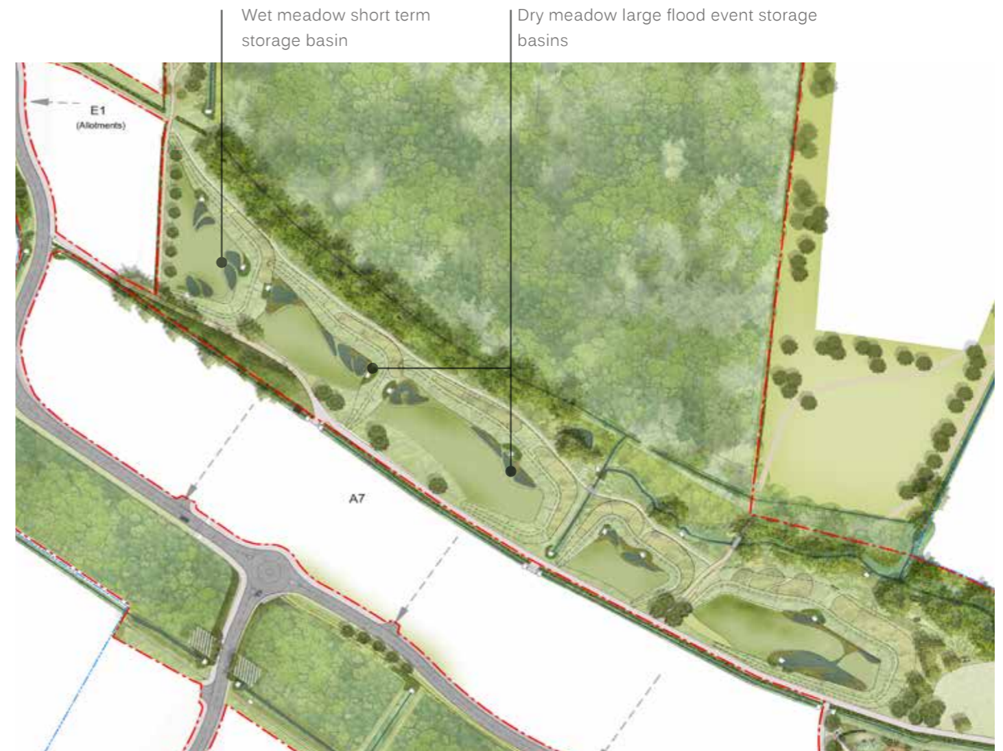
Figure 17. Stormwater Basins Extract from General Arrangement Plan
