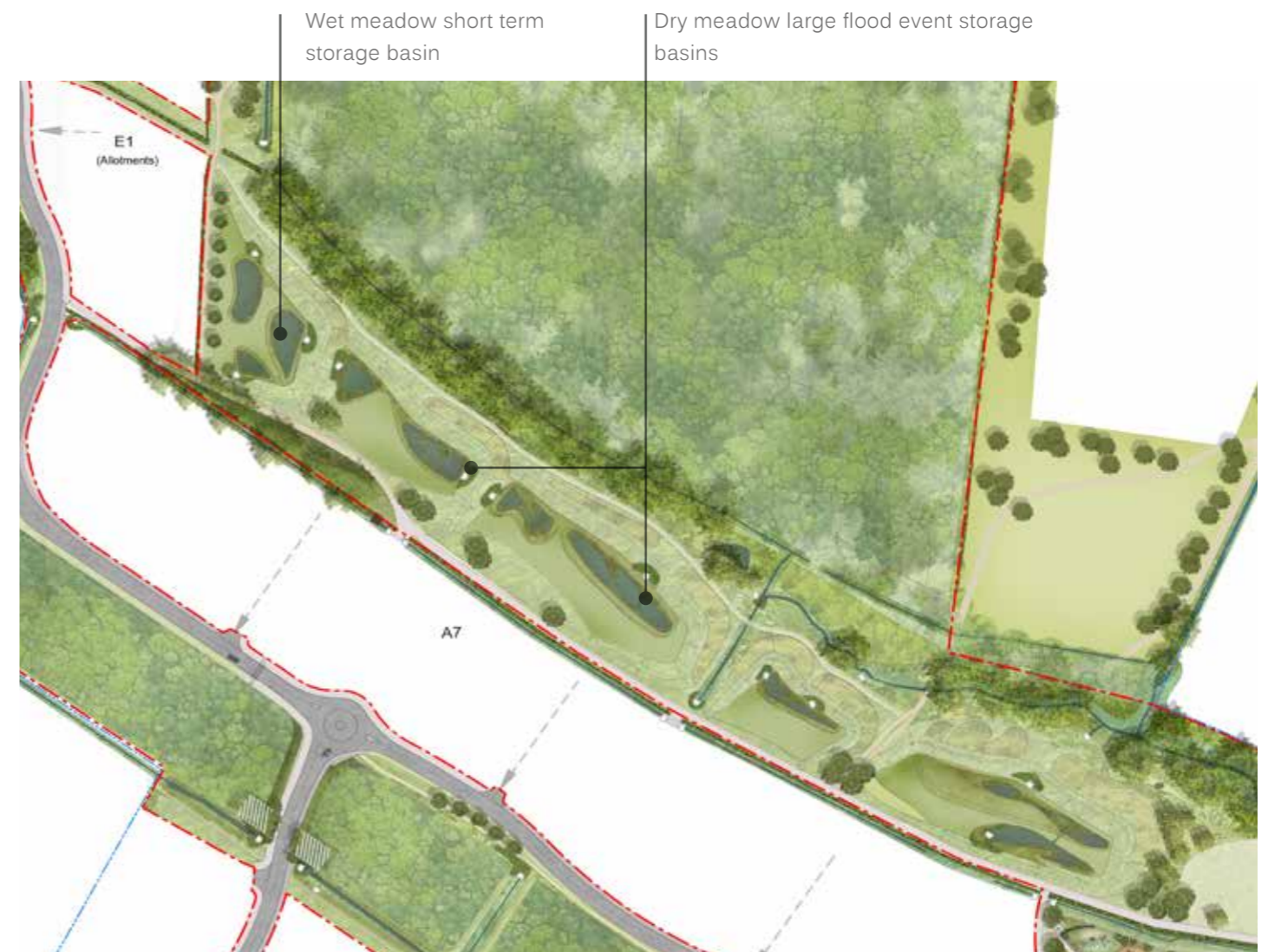
Figure 17. Stormwater Basins Extract from General Arrangement Plan
