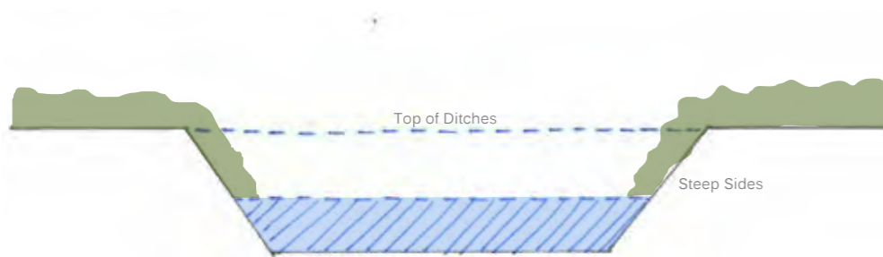
Figure 14. Typical Section Through Existing Drainage Ditch
