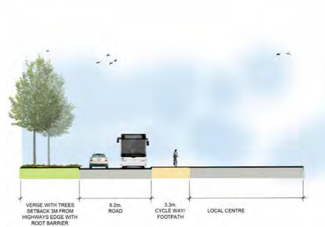
Figure 20. Section B - Through Northern Urban Centre (See Section 6.1 for Details on Bat Hop Over)
