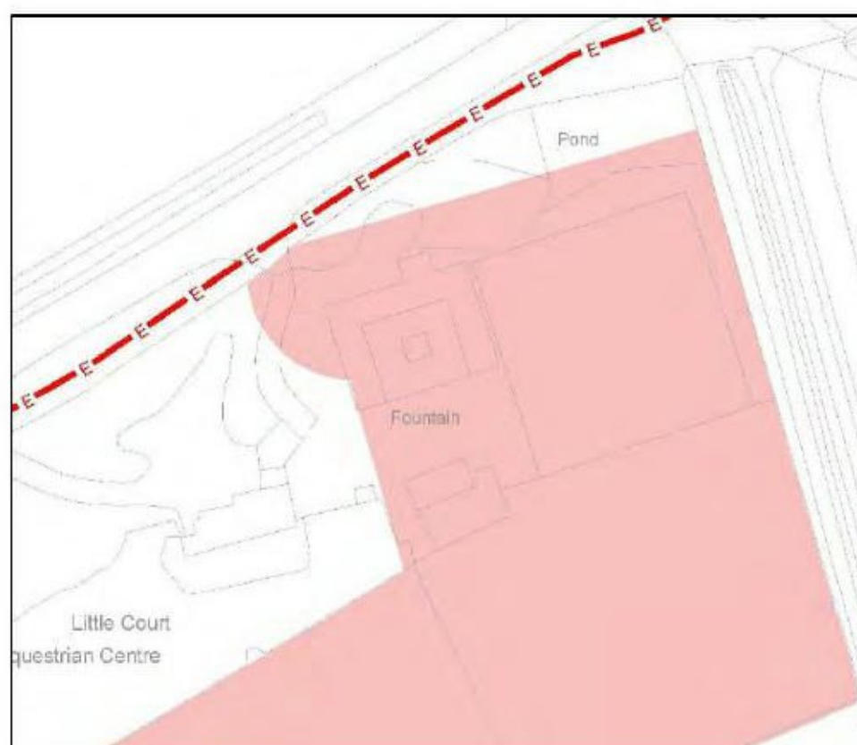
Figure 2 Existing UKPN infrastructure.
