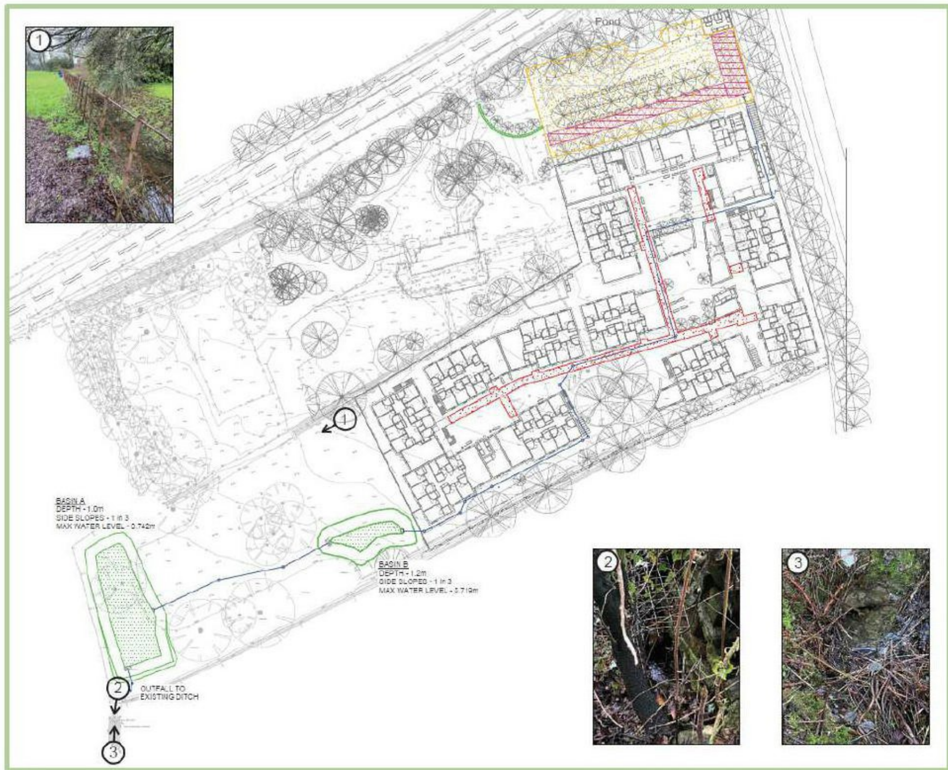
Figure 4.2 – Surface Water Management Strategy (Source: Cannon Consulting Engineers)
