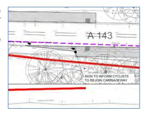
At the transition, cyclists will have difficulty viewing westbound approaching vehicles. The westbound traffic lane is narrowed by the presence of the central hatched markings and a merging cyclist may be vulnerable to collisions with vehicles at this point.
