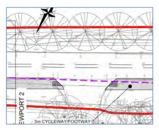
The driveway is shown as a fully kerbed access. It would appear to be a single property access and it may be appropriate to provide this as a dropped kerb crossover, to remove the need for tactile paving.
