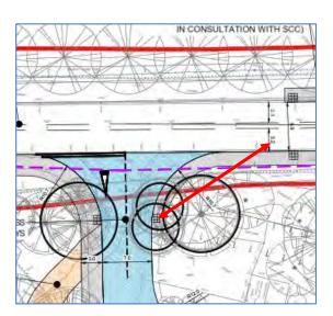
At the eastern footway crossing area, there may be reduced inter-visibility between pedestrians and drivers making the left turn in to the site. Reduced inter-visibility may lead to pedestrian to vehicle collisions.
