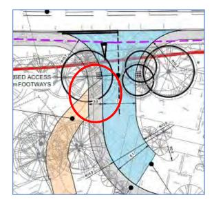
The private driveway is located close to the dropped kerb pedestrian crossover and the give way line. This may lead to occasional over-run of the tactile paving and possible damage to paving. It is suggested that the driveway access is relocated further from the crossing area, to provide separation; this would also increase the distance between the give way line and the access.
