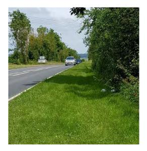
The A143, east of the development access, has a slight rolling vertical crest curve, with a raised verge area along the southern side of the A143. This may reduce the side road visibility to the right from the development access. Reduced side road visibility may lead to failure to give way type collisions, particularly as this section of the A143 is on a straight alignment and vehicle speeds appeared to be high.
