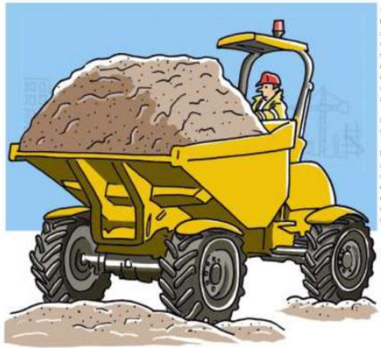
Figure 1. Example of unsafe dumper operations
