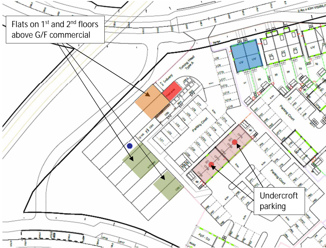
Figure 3. Proposed Local Centre external area layout. External G/F plant area shaded red, and receptor groups closest to plant area other colour-shaded.
