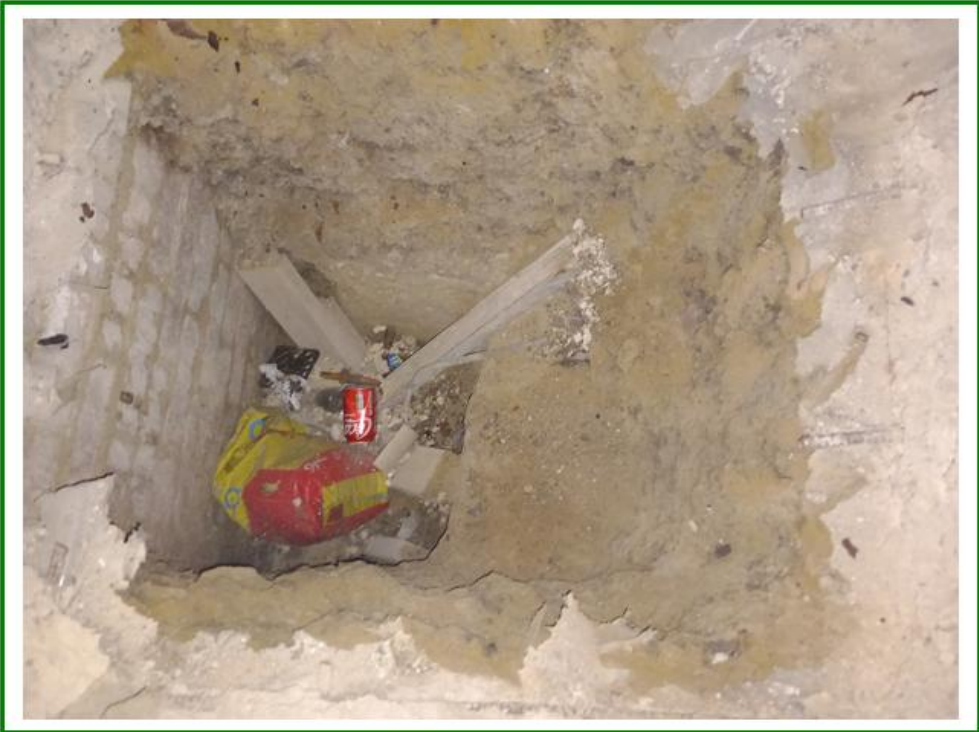
Photo No.21: Fourth inspection pit noted within the structure showing limited made ground deposits atop gravelly sands
