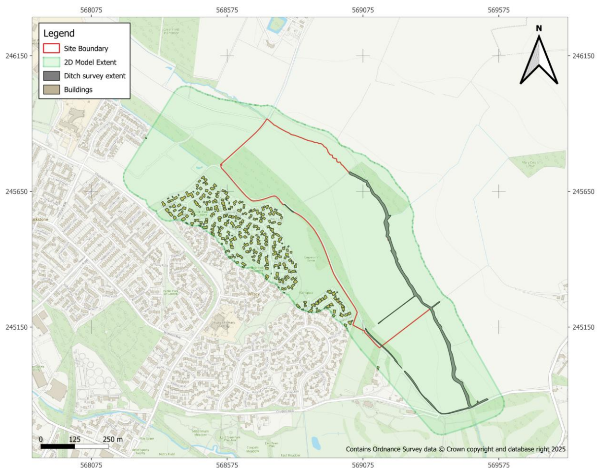
Figure 4 – Buildings and ditch extents used for DTM modification.
