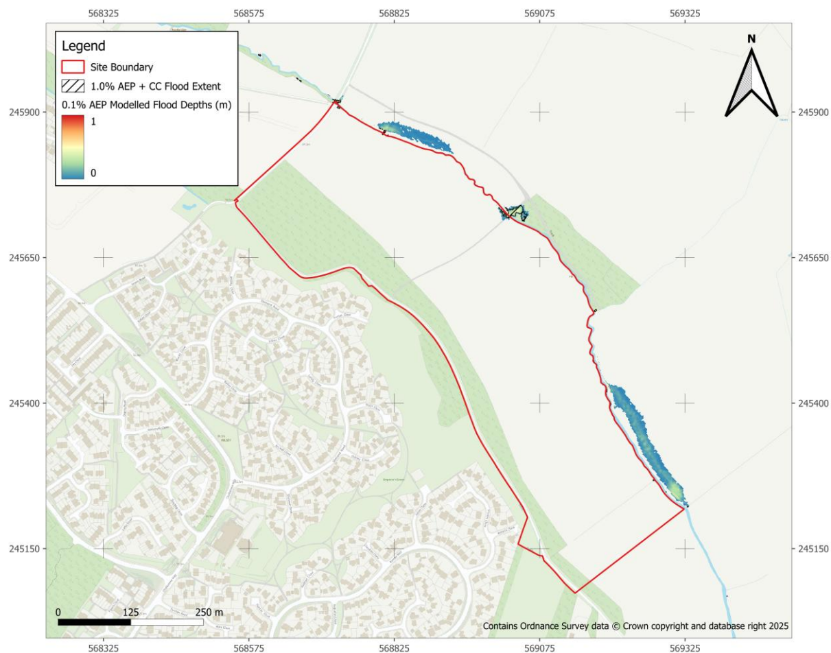
Figure 11 – Post-development model results for 1.05 m culverts (Option 1)
