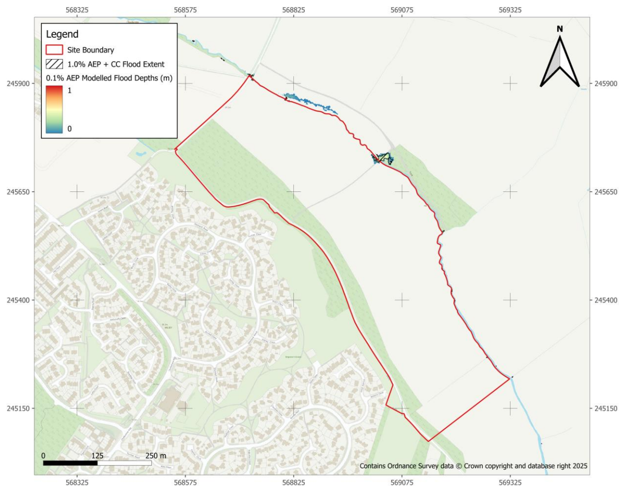
Figure 13 – Post-development Results for 1m x 1.5m box culvert (Option 2)
