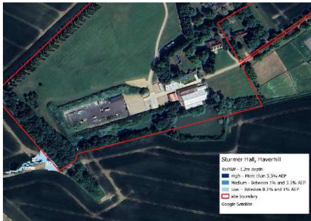
Figure 16- RoFSW Depth 1.2m
