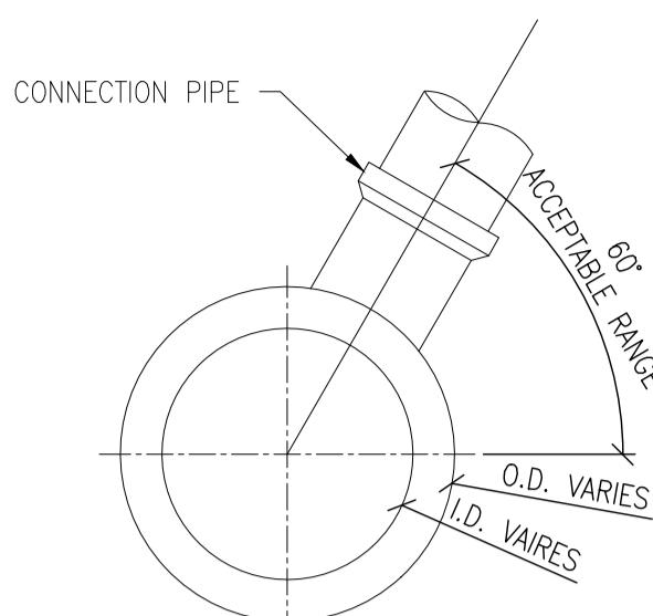
CROSS-SECTION VIEW OF SADDLE CONNECTION
