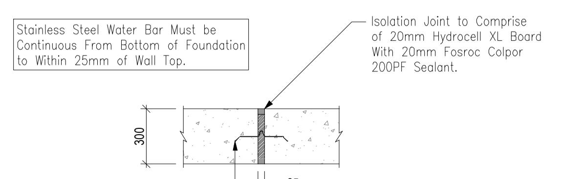
Typical Bund Wall Movement Joint Detail
