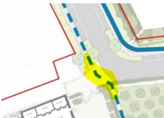
This part of the site will provide a vehicle turning head that will be used by refuse collection vehicles. The red circle in the snip below shows that there will not be a radius on the southern kerb line. Because this section of road is to be used for vehicle turning, this layout may be inconvenient and lead to kerb damage.
